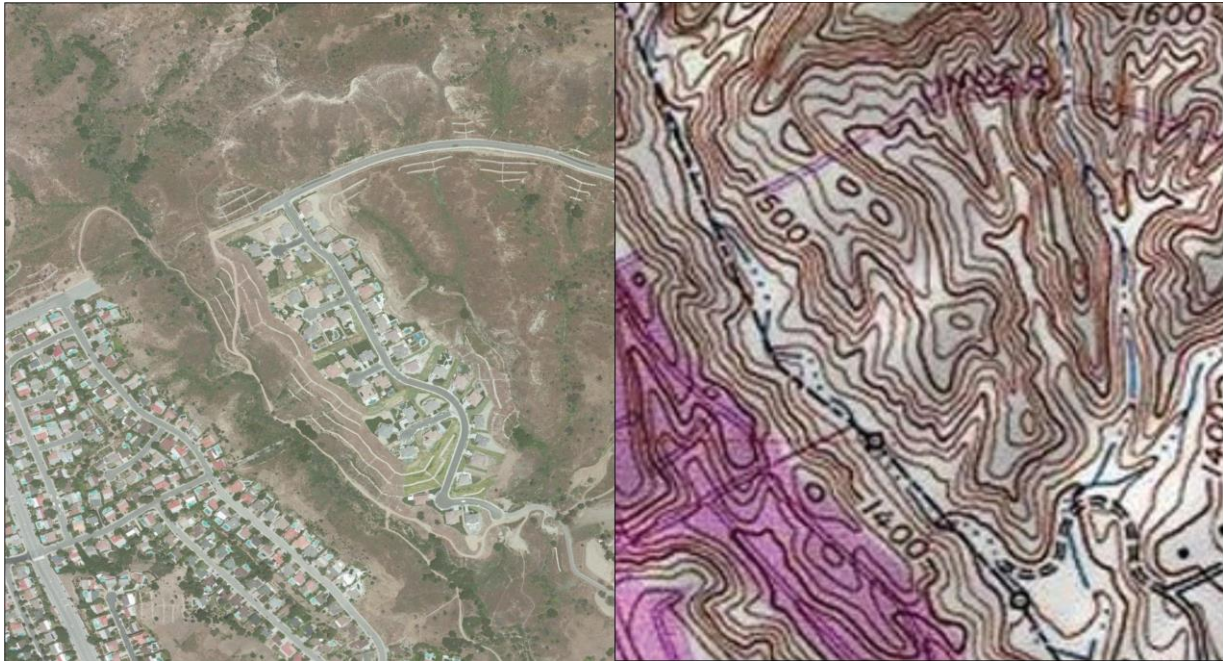
Figure 5.3: Common Raster Graphics Used in GIS Applications: Aerial Photograph (left) and USGS DEM (right) (Source: Data available from U.S. Geological Survey, Earth Resources Observation and Science (EROS) Center, Sioux Falls, SD.)
